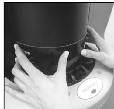
Figure 9 A Panoramic Plate being fed into the ScanX
