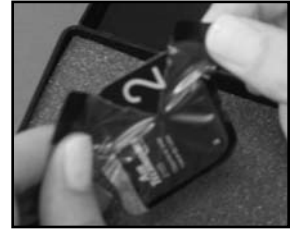
Figure 4 Ejecting a Plate into the Plate Transfer Box
