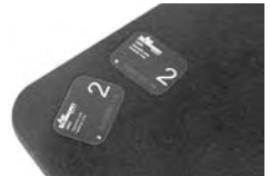
View C PSPs ready for Scanning
