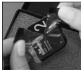
Figure 5 Ejecting a Plate into the Plate Transfer Box
